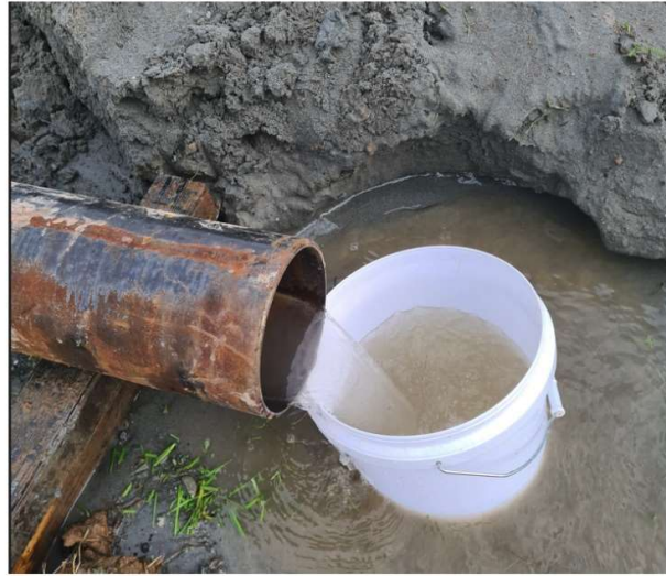
Figure 23: Ad hoc collection of direct injection water bypass / seepage for measurement with a 10 litre bucket
