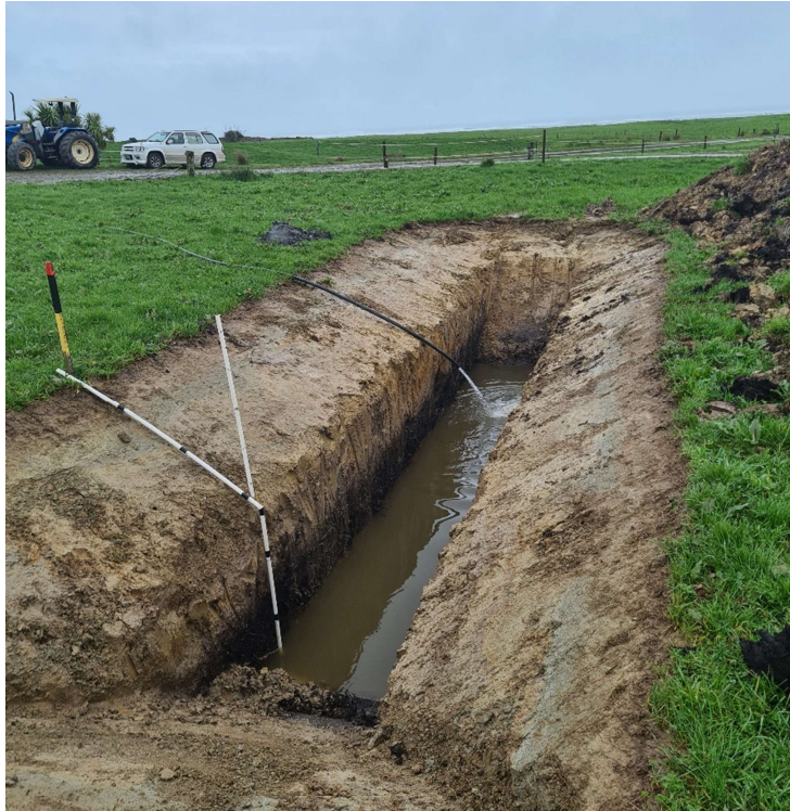
Figure 24: Water level in infiltration trial trench during initial filling, vegetation layer visible as darkened material above water level
