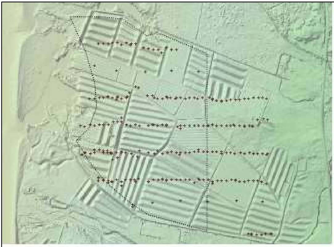
Figure 33: Location of TAC-### reverse circulation drill holes from 2022 (dotted line indicates mining area)
