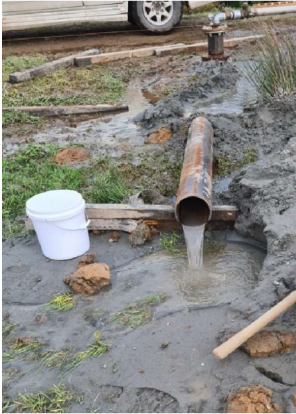
Figure 23: Ad hoc collection of direct injection water bypass / seepage for measurement with a 10 litre bucket
