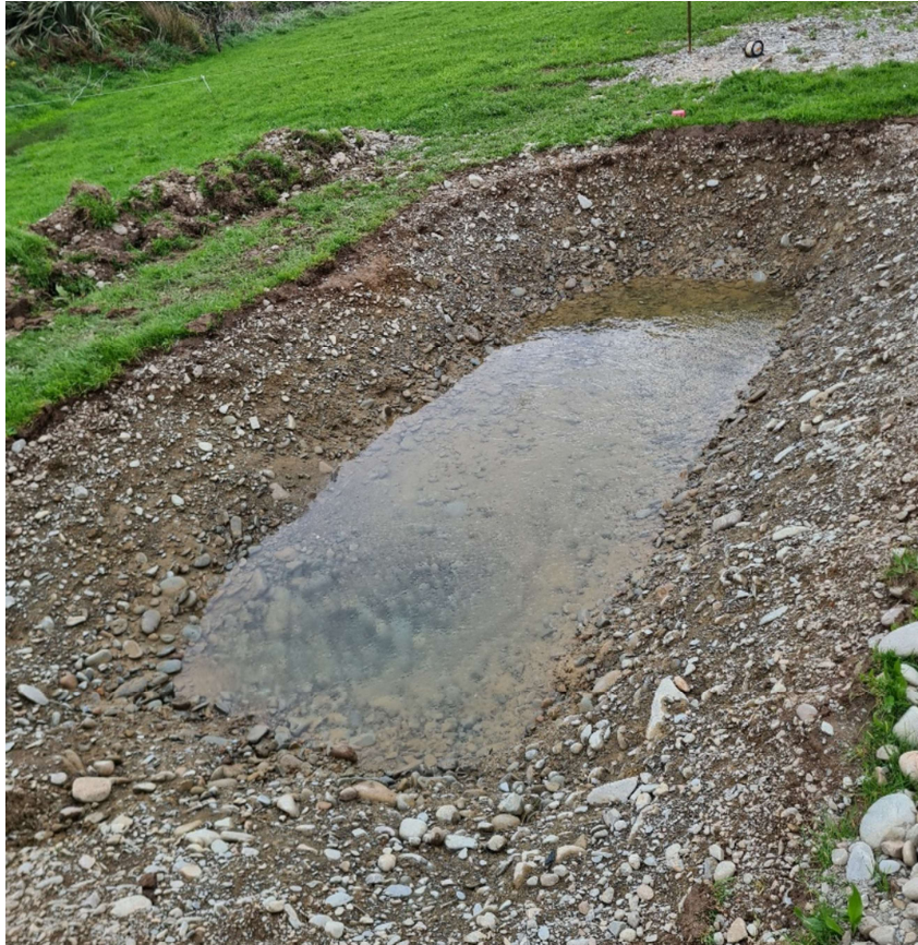
Figure 32: Draining infiltration trench 30 minutes after the cessation of infiltration (piezometer in background)
