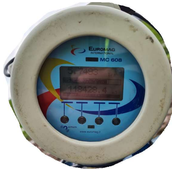
Figure 17: Mag-flow water flow meter used to measure injection rate, showing 5.7493 L/s injection
