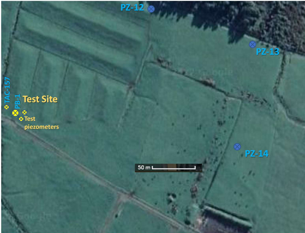
Figure 3: PB-1 test sit, including three observation bores (piezometers) in an area with known alluvial sediments
